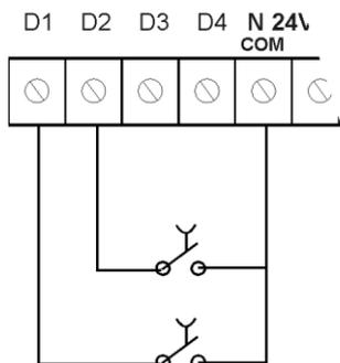
A time for the detection delay can be configured for every input, but deactivation is immediate.
