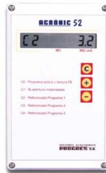
Device which blends in continuously the two waters to obtain a programmed conductivity, by using one or two motorized valves.
