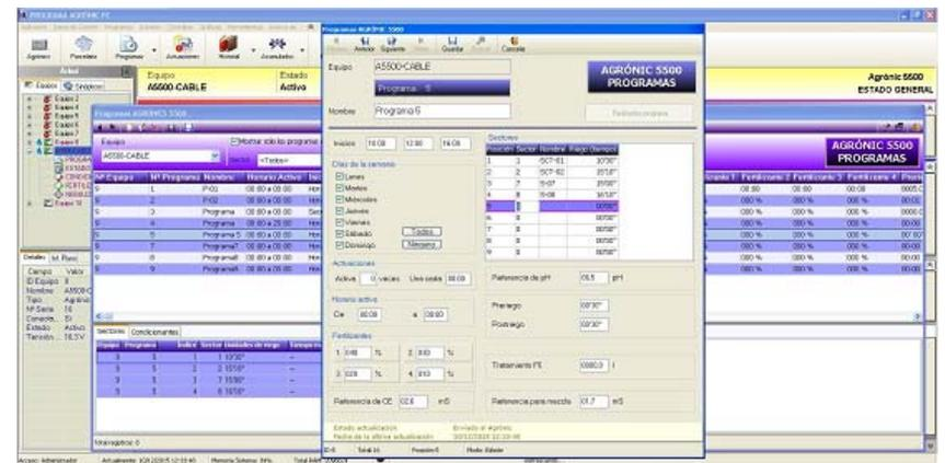
The Agronic 5500 manages the communications with three users; the data modified by a user is automatically updated on the other two. The connection of these three to the set can be simultaneous or permanent, depending on the link used. It can be used, for example, to interact with the proprietary, the allotment manager and the installer.
