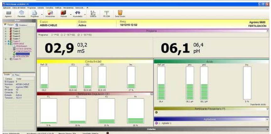
From the AGRONIC PC it is possible to obtain detailed information about the programmer (history, incidents, irrigation conditions, etc.) being able to act in order to modify parameters, programs, ranges, etc., from any place through a PC. The connection can be permanent and grouped alongside other controllers (Agronic 7000, 2500, 4000, BIT).
