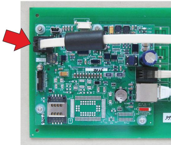
6. Cables disconnected in point 3 must be connected back again. Place the keyboard in the box and **move the new installed cable to the upper side of the box, avoiding it to directly pass over the main board and the keyboard.**
