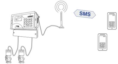
The Agrónic 2500 can send SMS when an event occurs in the equipment, with all 51 events being configurable. It also can send messages concerning all 30 determining factors. Every time the user sends a message to the Agrónic 2500 from their mobile phone, they will receive a response or confirmation message.
