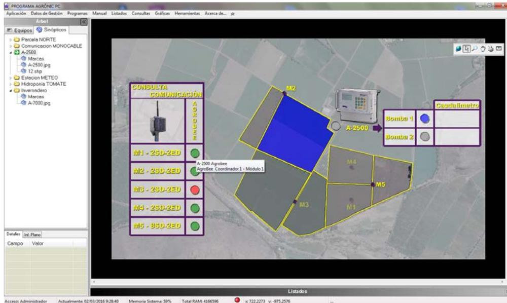
From the AGRÓNIC PC, punctual information can be obtained from the controller (history, incidents, irrigation situation, etc.), with the capability to modify parameters, programs, ranges, etc., from anywhere using a PC. The connection can be permanent and grouped together with other controllers (Agrónic 2000, Agrónic 4000, Agrónic 7000, Agrónic BIT).
