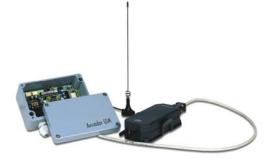
Avisador GSM is a unit designed to send SMS messages (text messages) to GSM mobile phones, once the signal from any external elements to which it is connected is received. It can be used with any system which needs to send warnings or alarms to mobile phones.
