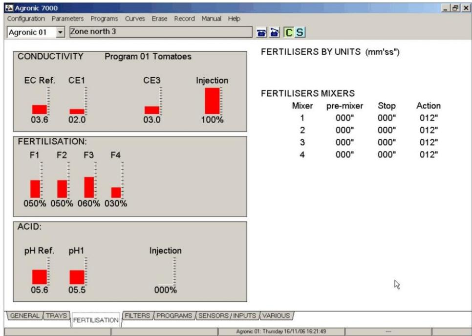
Injection of acid (pH): it displays the columns of desired acid reference, the reading of the main sensor (pH1) and the reading of the security sensor (pH2) and the % of injection of acid. It also indicates whether acid 1 or acid 2 or base is being injected.
