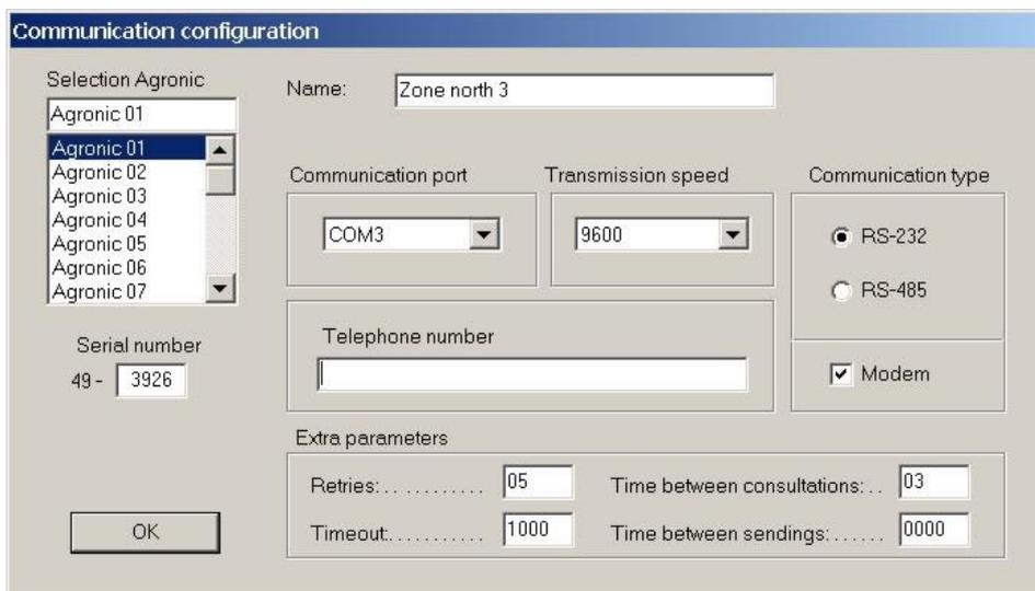
The number of Agronic must correspond with the one entered in the unit in the section of “Parameters – Configuration – Communication”.
