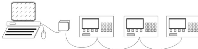
**Option C:** For equipment where the connection of the PC with the Agrónic is done by telephone (conventional modem or GSM) and every Agrónic has its own telephone line. Select the type of communication RS-232 and modem. For this type of communication we need a modem for the PC and a modem for every Agrónic to be connected.
