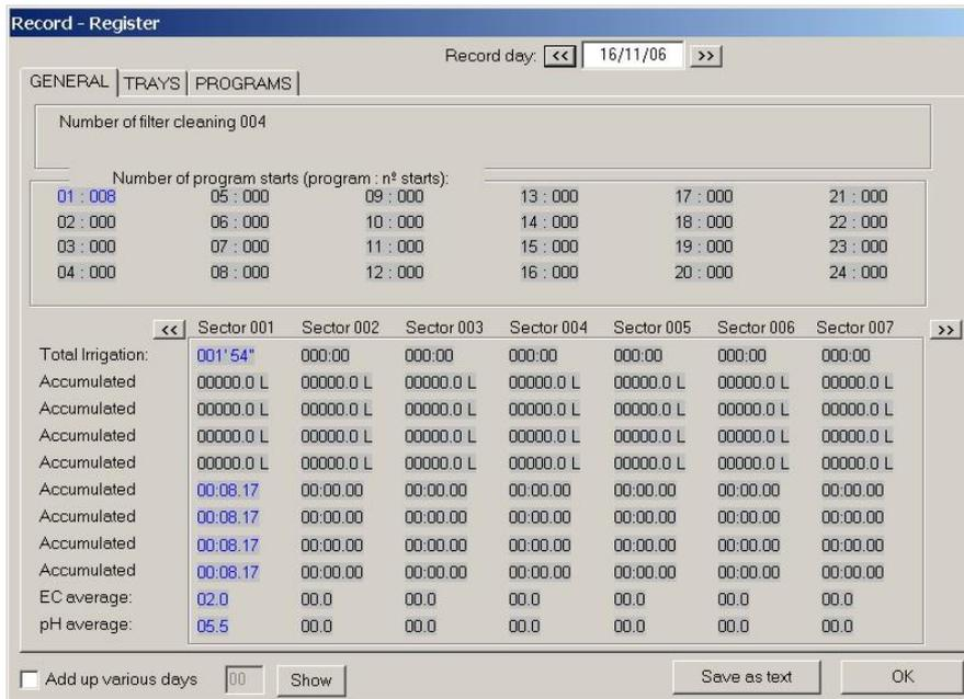
In the PC record there is one more field than in the Agrónic 7000, the one of "Programs" where a graphic shows what time and which programs have been started up during the day. If you place the mouse on the point which indicates the start of the irrigation values at the upper part of the dialogue, the values of program start are displayed. With the button of "+ Zoom" the graphic shows the period of time between 8 a.m. and 8 p.m. allowing you to see more accurately program starts.
