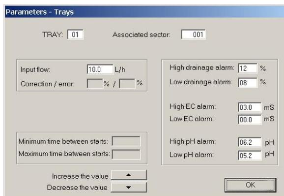
**2.- Parameters - Flow.** To determine the working units, both for the irrigation and the fertilization, as well as the high and low margins which an alarm will generate.
